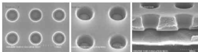
Residue removal from MSQ ILD vias as compared to Figure 4 (no clean).
