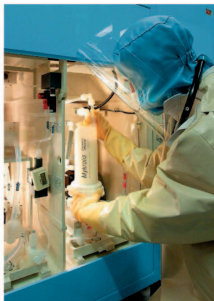
Typical filter installation within a process tool.
